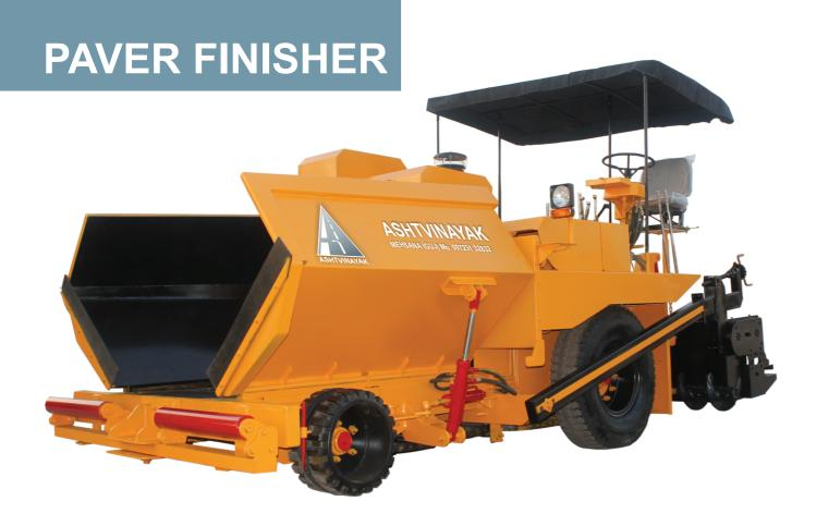
WM-6 HES is fitted with a power steering for ease of operation, a 105 HP @2000rpm engine for enhanced power and oil disc brakes. The bearing pedestral is protected form dust. The Hydraulic extension are eliminated and the screed width can be easily varied between 2.5 M to 4.5 M hydraulically
